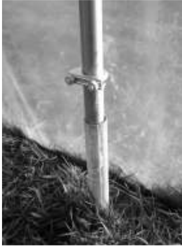
Raising the hoop (and clamp) to tension cover.
