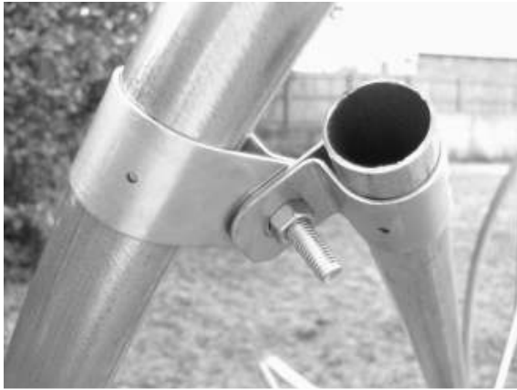
*Correct clamp position - Inside the end hoop.
